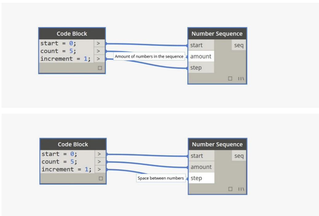
Figure 11 To create the array of points, the user must first create a number sequence. It might be preferable to use the more precise term 'length' rather than the more ambiguous term 'amount' and to use the more precise term 'increment' rather than the terms 'step' and 'space'
