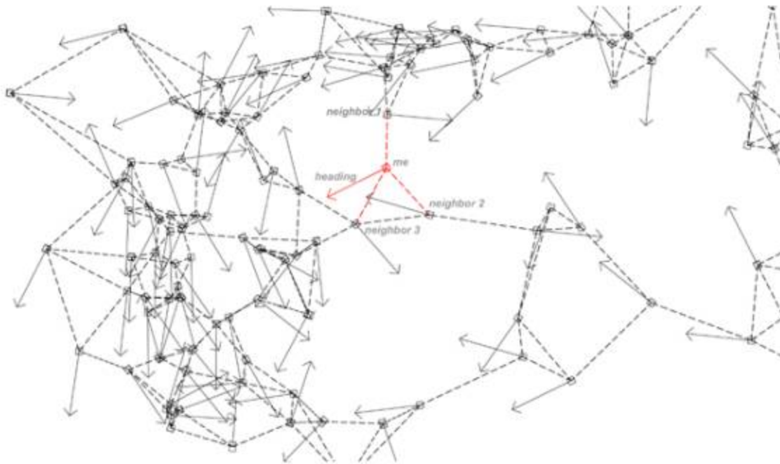
Diagram of the swarm. Arrows represent each agent's heading, dotted lines their closest neighbours.
