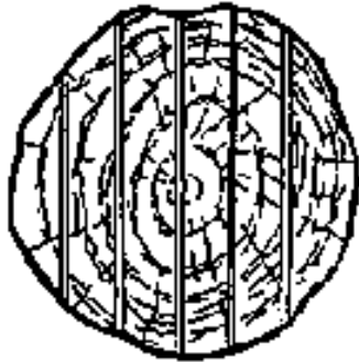
The log goes through the circular saw while still held in one position.
