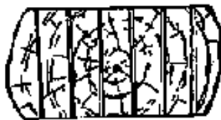
The log passes through the saw in two separate operations. Firstly - Slicing the outside parts Secondly - Slicing the middle section.
