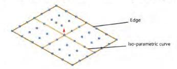
Each vertex on the surface can have a weight which "pulls" the surface towards the weighted vertices.
