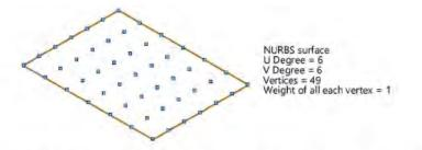
A NURBS surface also has a direction, or normal, which affects the outcome of certain operations, such as fillet surface creation. Iso-parametric curves indicate the U and V direction, and edge curves are drawn along the edges, helping to visualize the NURBS surface.
