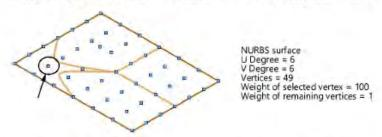
The Reshape tool can move a single vertex or a row of vertices, deforming the surface (see Reshaping NURBS surfaces)
